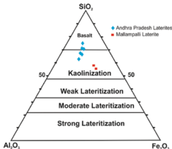
Figure 4. The Mallampalli laterite fall on the Kaolinization field and AP laterites fall on the basalt field in the Ternary diagram (SiO 2 -Fe 2 O 3 -Al 2 O 3 ) (Schellman, 1981).
