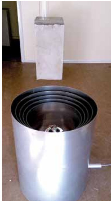
Figure 6. Interior view of mu-metal shield pictured without lid
