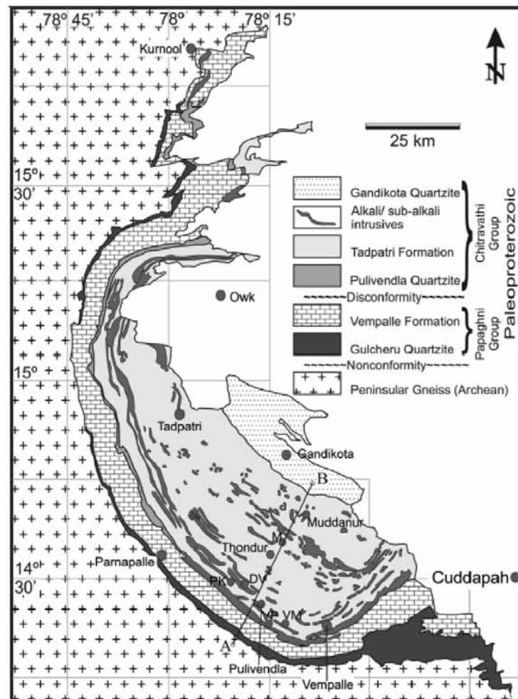
**Figure 2.** Geological map of SW part of the Proterozoic Cuddapah basin. Note the mafic-ultramafic sills disposed parallel to the basin configuration along its western margin. Section A-B from western margin of the basin- Pulivendla-Tonduru-Muddanuru-Gandikota transcends through Papaghni and Chitravathi Groups. Abbreviations: DV- Dondlavagu; M- Mallela; PK- Peddakudala; VM- Vemula; VP- Velpula
