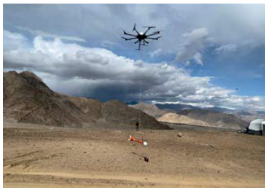
Drone based Magnetic Survey in Ladakh
