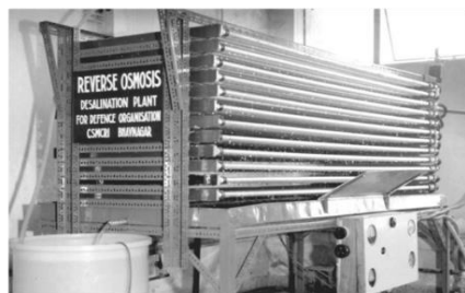
CA based tubular RO desalination plant Capacity 10,000 LPD : Jodhpur
