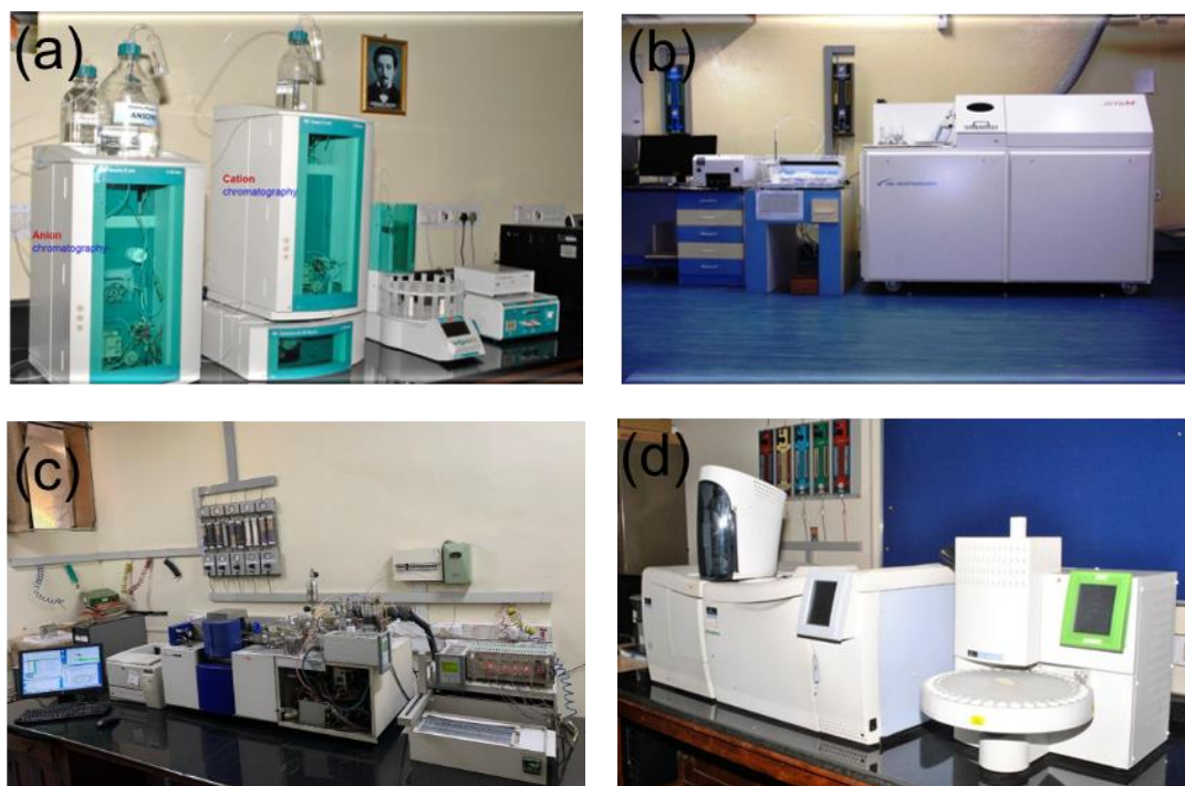
Figure 7. Laboratory facilities for hydrogeochemical investigations for geothermal exploration. (a) Ion Chromatography with Autosampler for Major anions and cations, (b) High Resolution-Inductively Coupled Plasma Mass Spectrometer (HR-ICP-MS) for Trace Elements and REEs, (c) Isotope Ratio Mass Spectrometer (IRMS) for Stable isotopes, (d) Gas Chromatograph-Mass Spectrometer (GC-MS) for gases.
