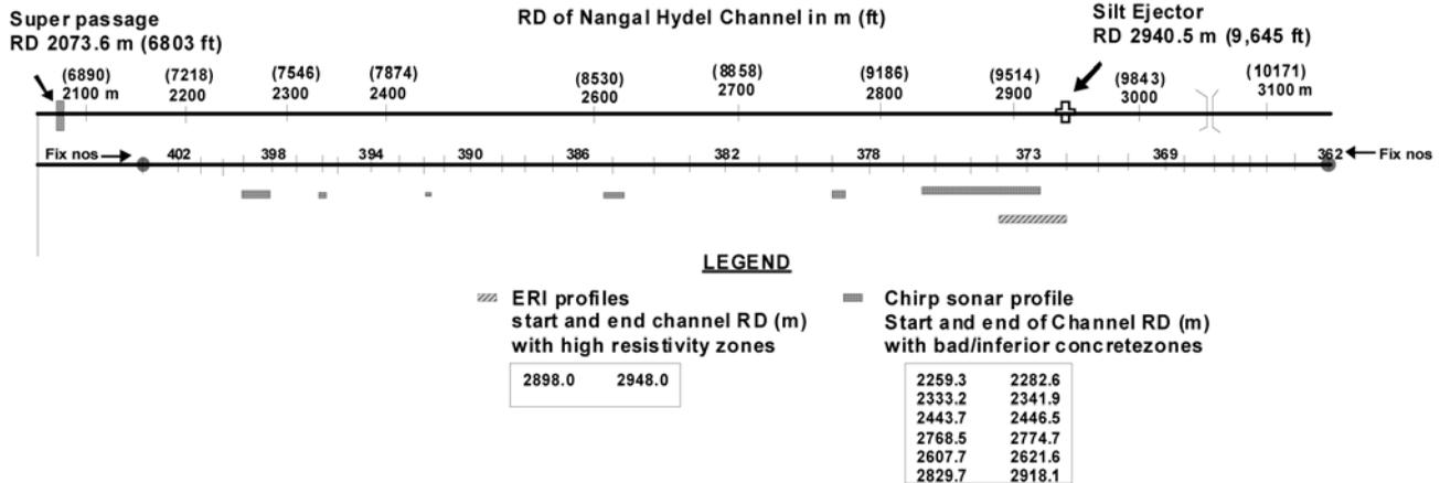
Figure 7. Nangal Hydel Channel RDs showing patches of bad and inferior quality concrete
