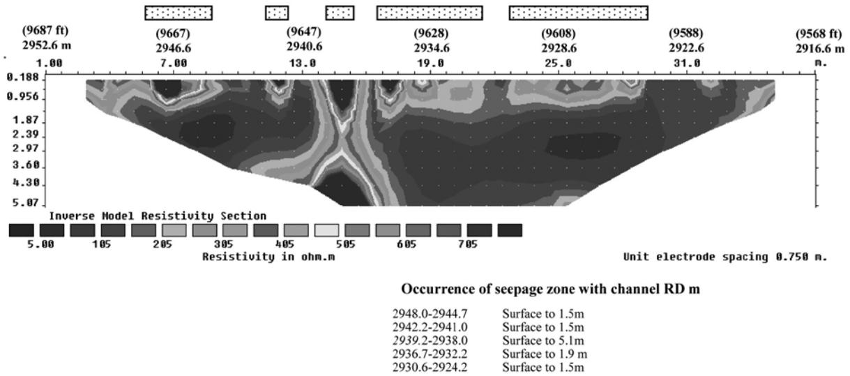
**Figure 6a.** Resistivity imaging section showing susceptible seepage zones at Silt Ejector site (Channel RD 2952.6 m – 2916.6 m)
