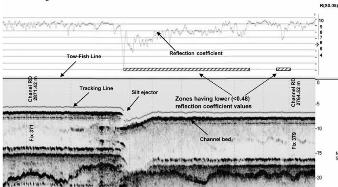
**Figure 5.** Typical Chirp Sonar Record Showing continuous graph of Reflection Coefficient values
