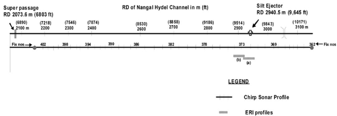
Figure 2. Schematic plan showing chirp sonar and ERI traverse
