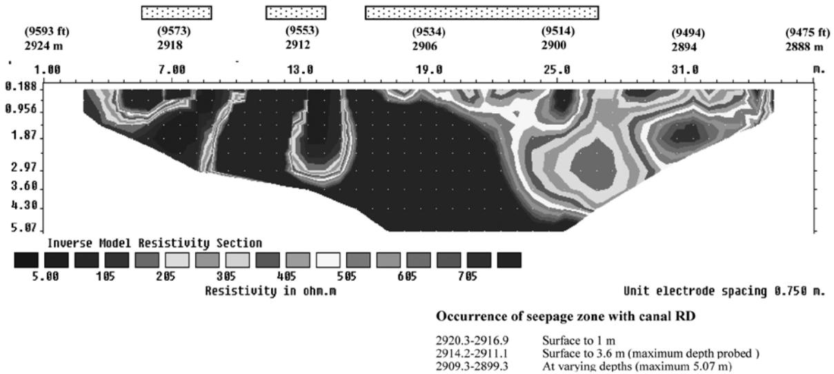
**Figure 6b.** Resistivity Imaging section showing susceptible seepage zones near Silt ejector site (Channel RD 2924 m - 2888 m)
