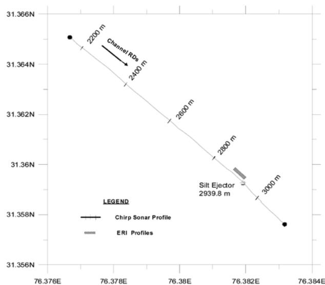
Figure 3. Layout of chirp sonar and Electrical Resistivity Imaging Profile
