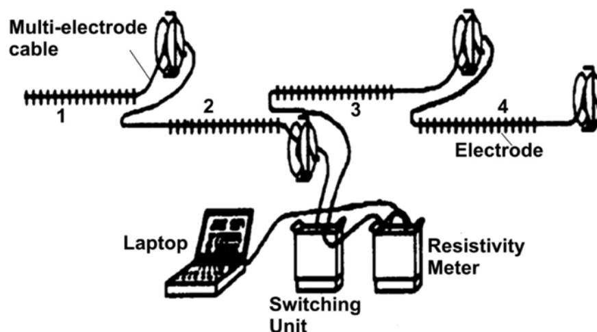
Figure 2. Field arrangements of ERT survey with 4 multi-core cables
