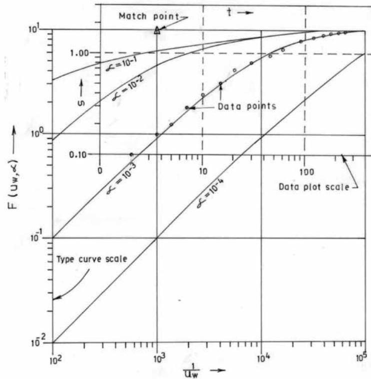
Figure 2. Analysis of pump-out test curve by matching of time-drawdown data of large diameter well (W1) with Papadopoulos-Cooper type curve.
