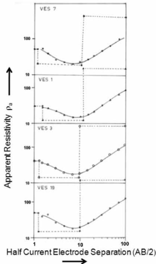
**Figure 3.** Typical sounding curves where the pump-out tests were carried out
