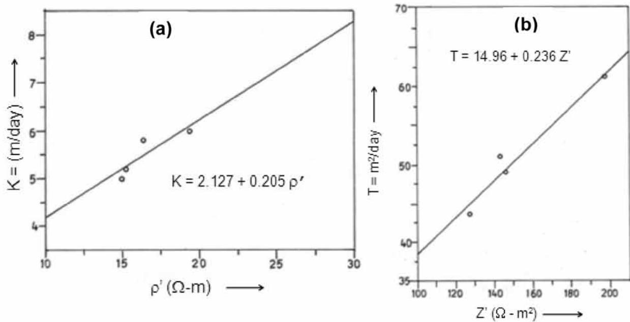
Figure 4. Correlation curves of: (a) K Vs  $\rho'$  and (b) T Vs  $Z'$
