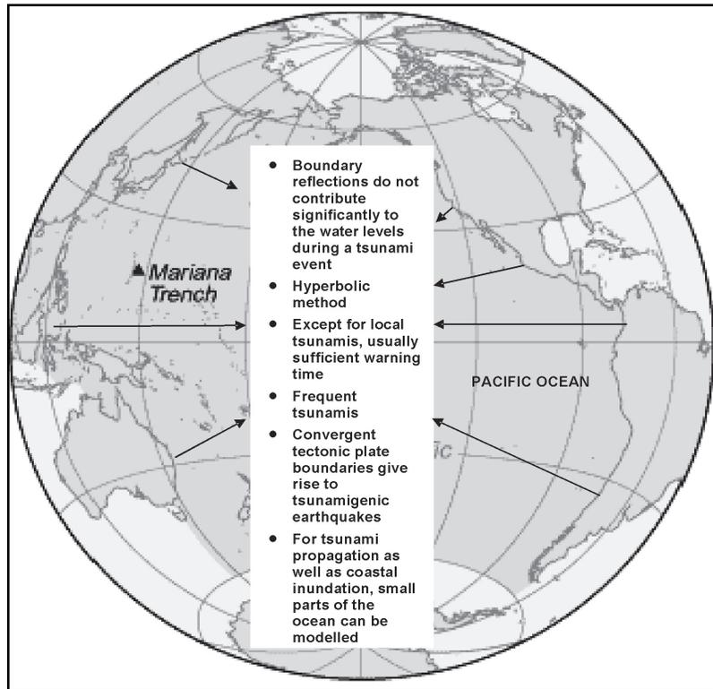
Figure 8. Schematic illustration of the tsunami numerical modelling concept for the Pacific Ocean
