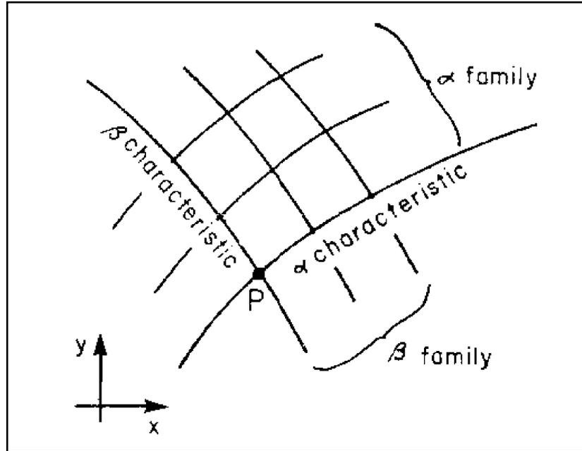
**Figure 7.**  $\alpha$  and  $\beta$  characteristics in a given domain. The slopes of the characteristics are  $(dy/dx)_a$  and  $(dy/dx)_b$ , respectively. (Crandall 1956)
