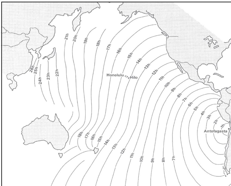
**Figure 3.** A tsunami travel time chart for the Pacific Ocean. The contours are in hours
