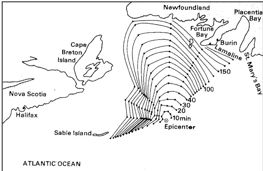
**Figure 4.** Tsunami travel times for the Grand Banks earthquake of 18 November 1929 (Murty 1977). The contours are in minutes.
