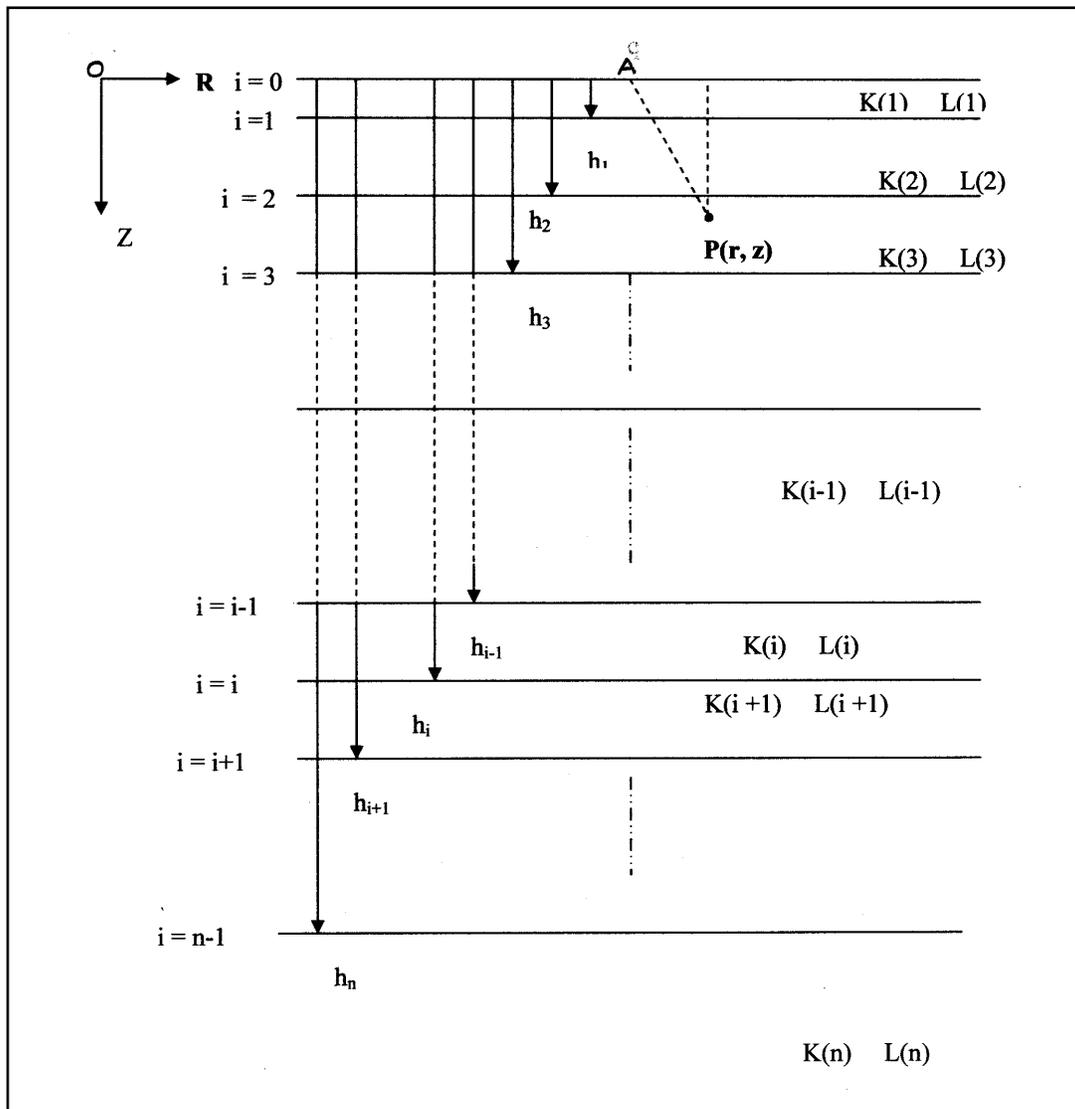
**Figure 1.** Schematic diagram for the multi-layered aquifer system with a point source at A;  $P(r,z)$  is any arbitrary point in the cylindrical coordinate system.
