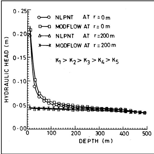
**Figure 6.** Vertical distribution of hydraulic head obtained from NLPNT (solid line) and MODFLOW (dashed line) at the source and at a distance 200m from the source for the 5-layered aquifer system with  $K_1 > K_2 > K_3 > K_4 > K_5$ .
