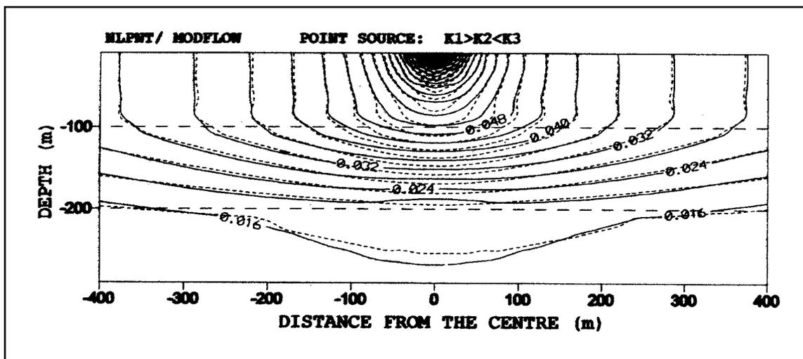
Figure 2. Equi-potential plot in the vertical section of a 3-layered aquifer system ( $K_1 > K_2 < K_3$ ) computed by NLPNT (solid contours) and MODFLOW (dashed contours).
