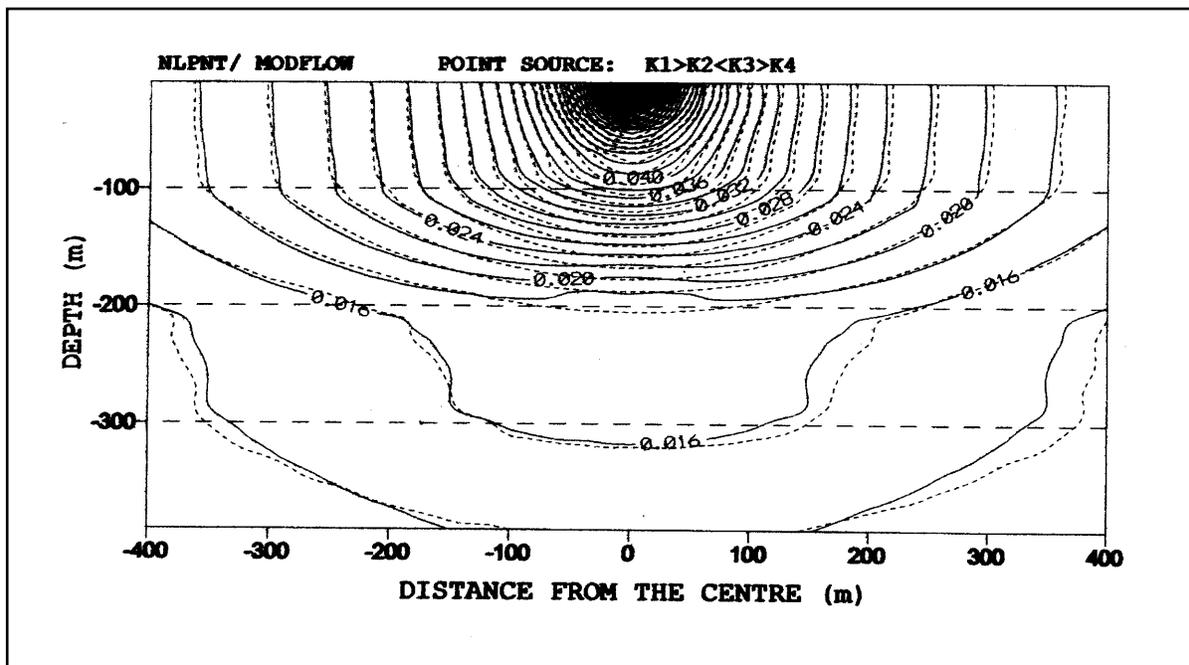
Figure 4. Equi-potential plot in the vertical section of a 5-layered aquifer system ( $K_1 > K_2 > K_3 > K_4 > K_5$ ) computed by NLPNT (solid contours) and MODFLOW (dashed contours).
