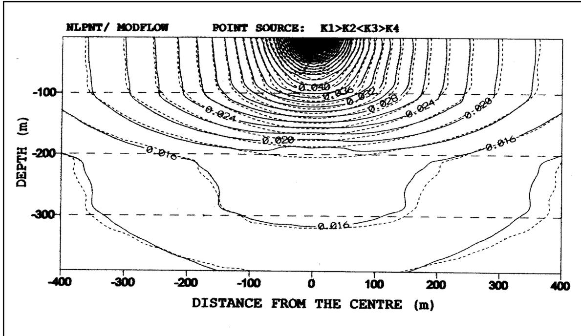
Figure 3. Equi-potential plot in the vertical section of a 4-layered aquifer system ( $K_1 > K_2 < K_3 > K_4$ ) computed by NLPNT (solid contours) and MODFLOW (dashed contours).
