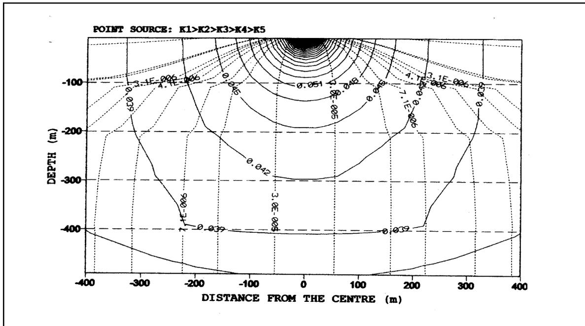
Figure 5. Equipotential plot (solid contours) and streamlines (dashed contours) in the vertical section of a 5-layered aquifer system ( $K_1 > K_2 > K_3 > K_4 > K_5$ ) computed by NLPNT.
