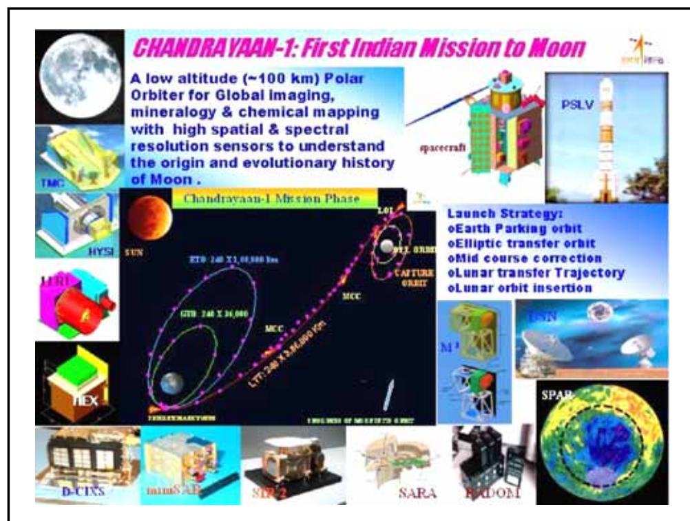
Figure 2. Details of Chandrayaan-1 mission showing different payloads to be launched for scientific investigations of lunar terrain, mineral deposits and trapped volatiles etc.
