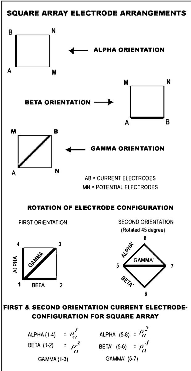
Figure 2. Electrode arrangements for square array (dc) resistivity method.
