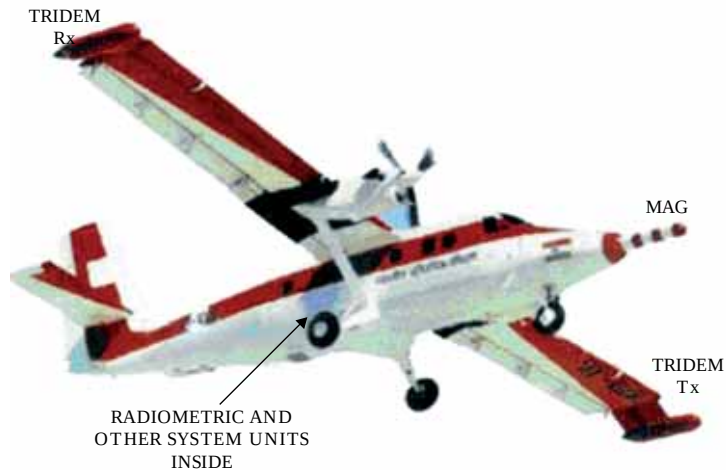
Figure 9. GSI's Twin Otter geophysical Survey System(from GSI's website)
