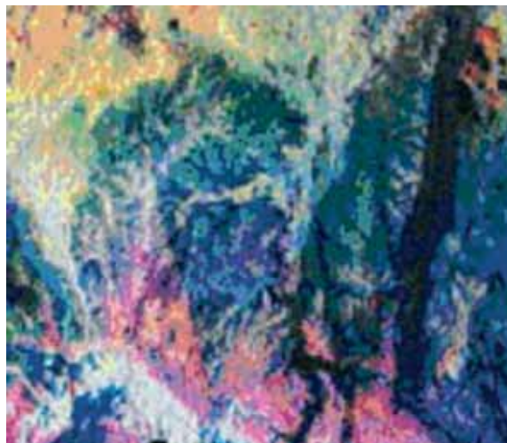
Figure 5. An example of ternary image of gamma-ray spectrometer data over an Archaean craton province
