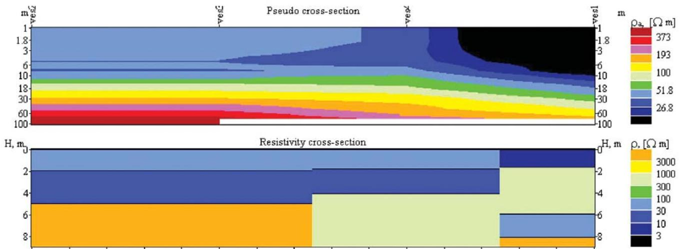
**Figure 5.** Pseudo cross-section and Resistivity cross section along the profile-I.
