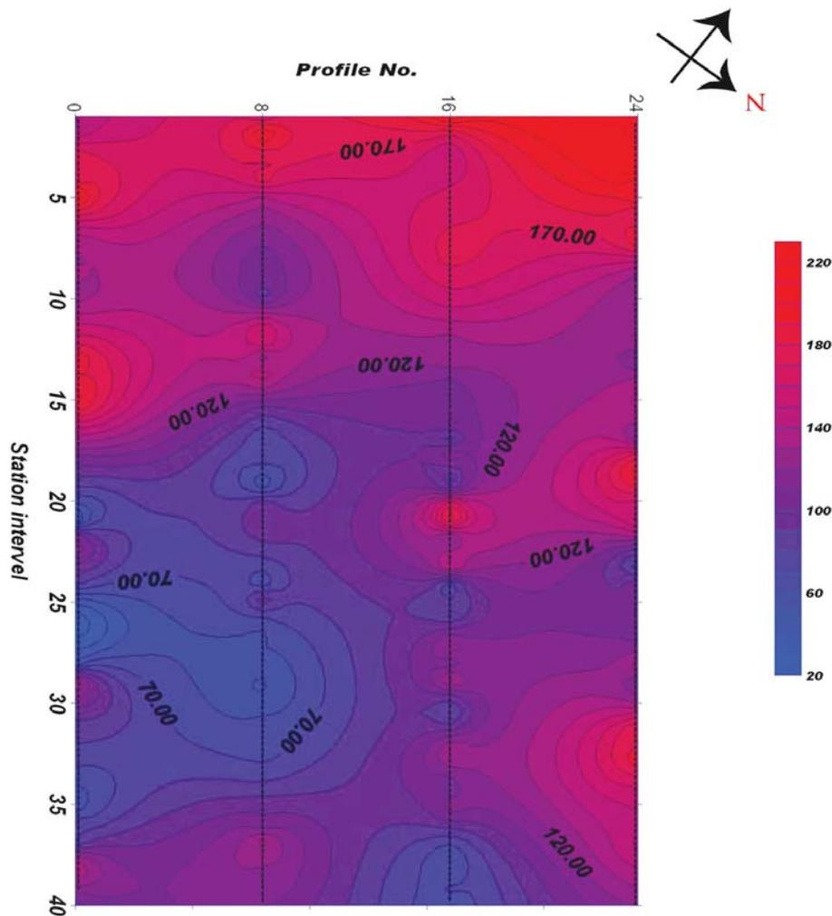
Figure 3. Contour map of the apparent resistivity.
