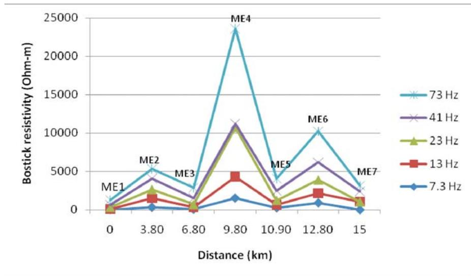
**Figure 3a.** Resistivity profiling curves for profile A (low frequencies).
