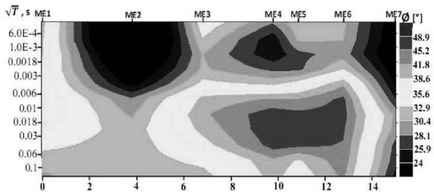
Figure 5b. Phase pseudo-section of profile A.
