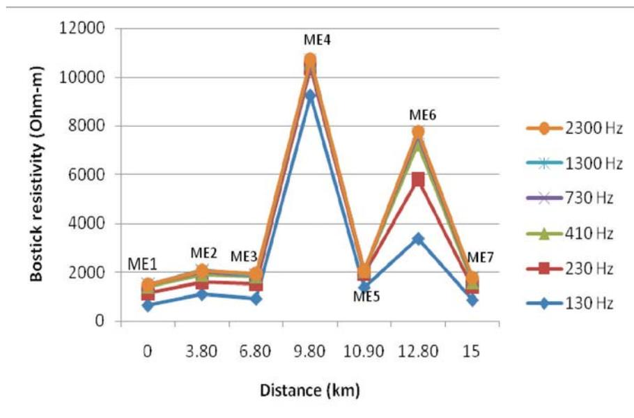
**Figure 3b.** Resistivity profiling curves for profile A (high frequencies).
