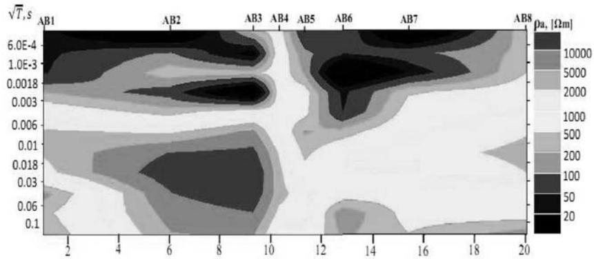
Figure 6a. Bostick resistivity pseudo-section of profile B.
