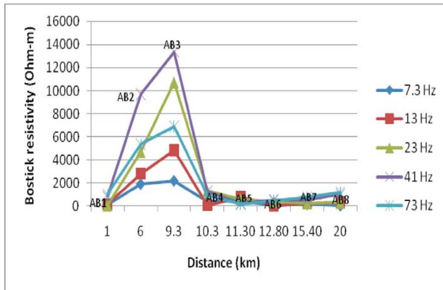
Figure 4a. Resistivity profiling curves for profile B (low frequencies).
