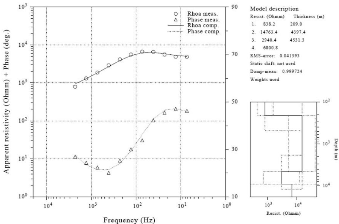
**Figure 2a.** Sounding curve illustrating a model of 4 layers (AB3 station).
