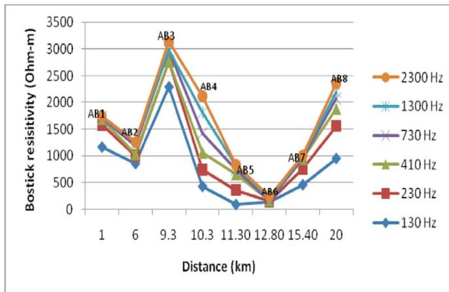
Figure 4b. Resistivity profiling curves for profile B (high frequencies).
