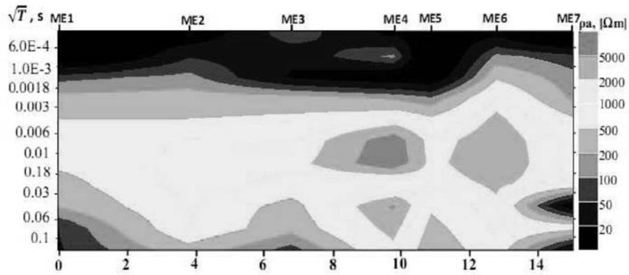
Figure 5a. Bostick resistivity pseudo-section of profile A.
