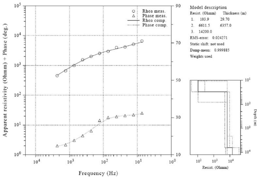
**Figure 2b.** Sounding curve illustrating a model of 3 layers (ME2 station).
