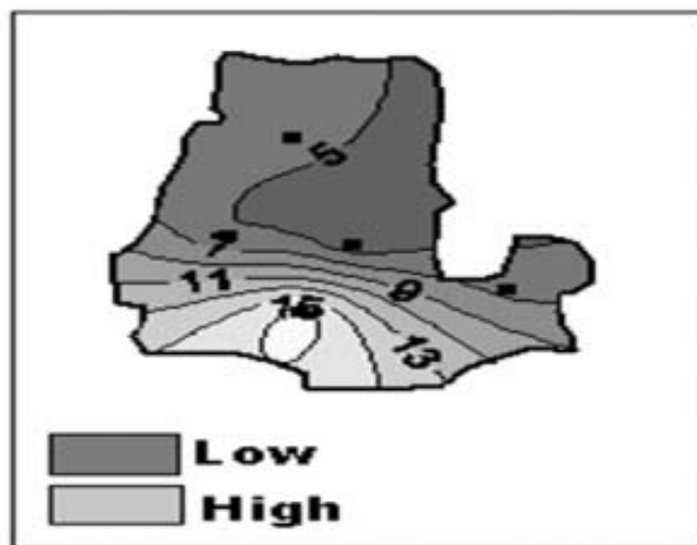
Figure 7. Iso resistivity map of Third layer.
