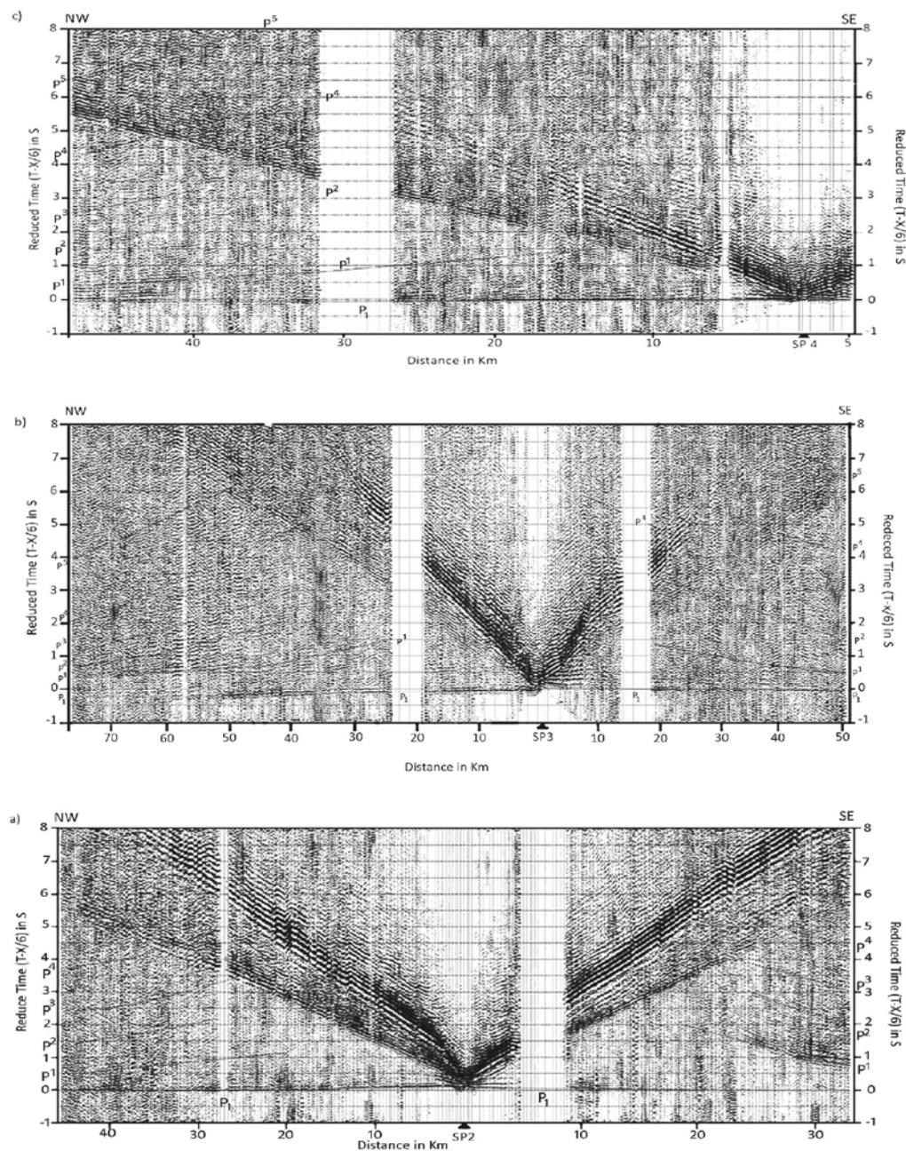
**Figure 5.** Shot gathers showing the first arrivals (P1) and various reflection phases (P1-P5) for (a) of SP2 (b) SP3 (c) SP4.
