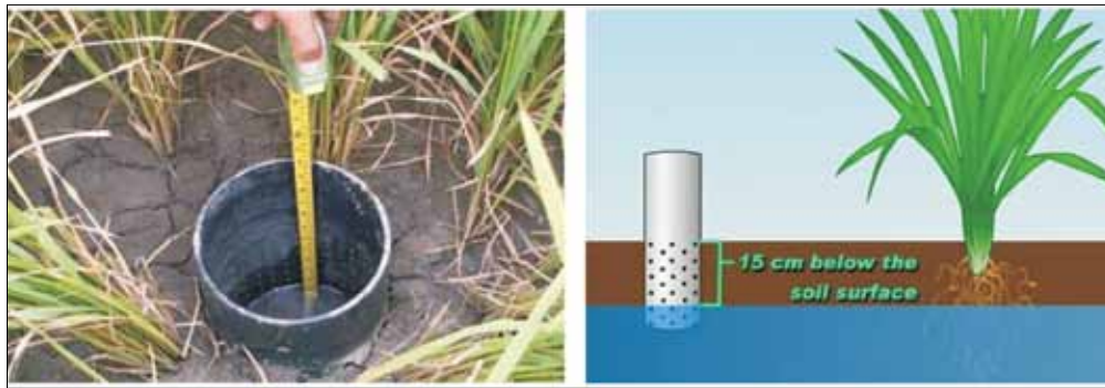
Figure 3. Panipipes used to monitor the water level in AWD method
