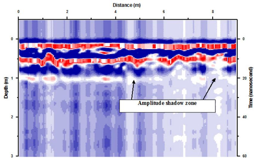
Figure 3. GPR record along profile P5 with amplitude shadow over oil contaminated zone
