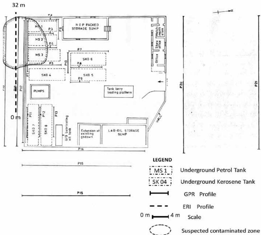
Figure 1. Layout of HPCL depot showing GPR and Resistivity Imaging traverses.
