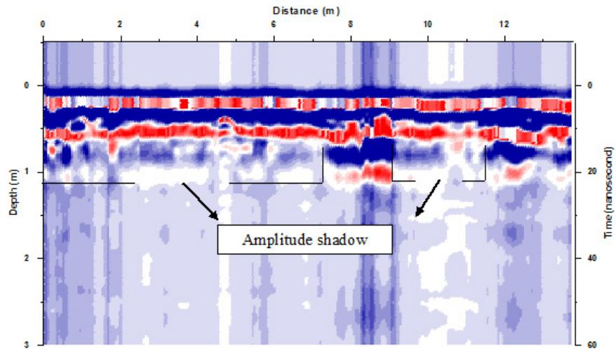
Figure 2. GPR record along profile P1 with amplitude shadow over oil contaminated zone
