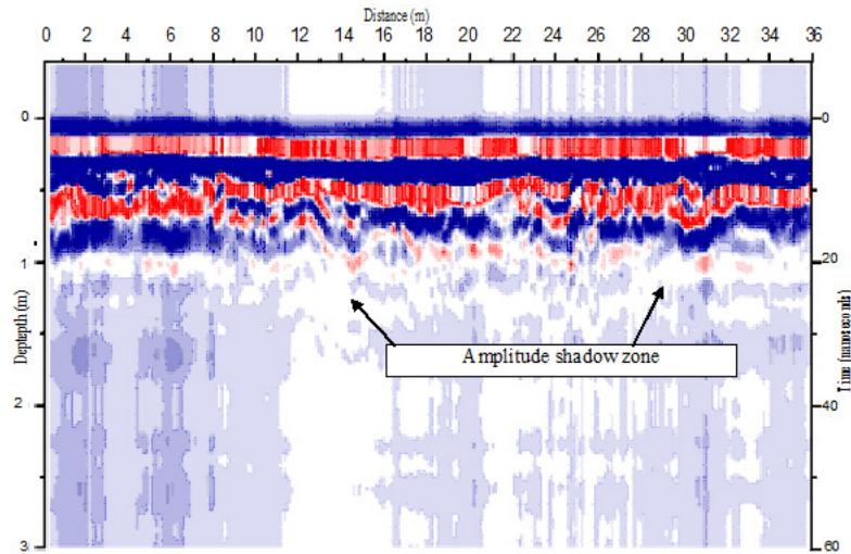
**Figure 4b.** GPR record along profile P17 with amplitude shadow over oil contaminated zone
