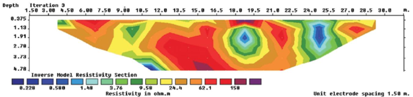
Figure 4a. Electrical Resistivity Image showing oil contaminated zone
