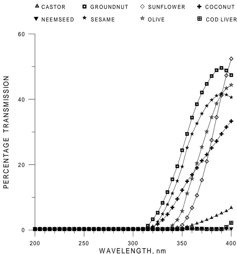
**Figure 1.** Percentage transmission of oils shown against wavelength obtained using a UV – VIS spectrophotometer. A quartz cell was used as the container for the oil.
