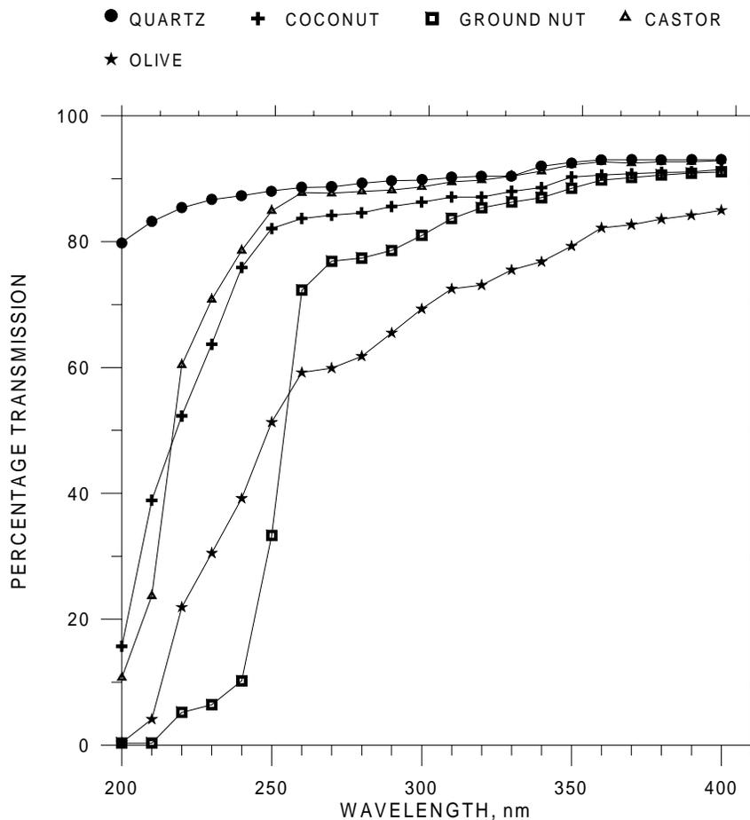
**Figure 2.** Percentage transmission of four oils shown against wavelength obtained using a UV – VIS spectrophotometer. The transmission of quartz disk used as the substrate is also shown.
