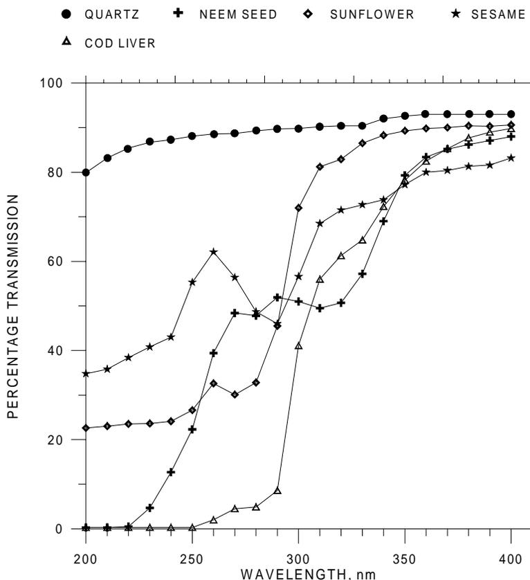
**Figure 3.** Percentage transmission of four oils shown against wavelength obtained using a UV – VIS spectrophotometer. The transmission of quartz disk used as the substrate is also shown.
