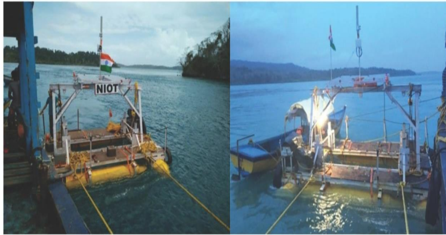
Figure 1. Hydrokinetic turbine testing at the Andaman Islands, India by NIOT
