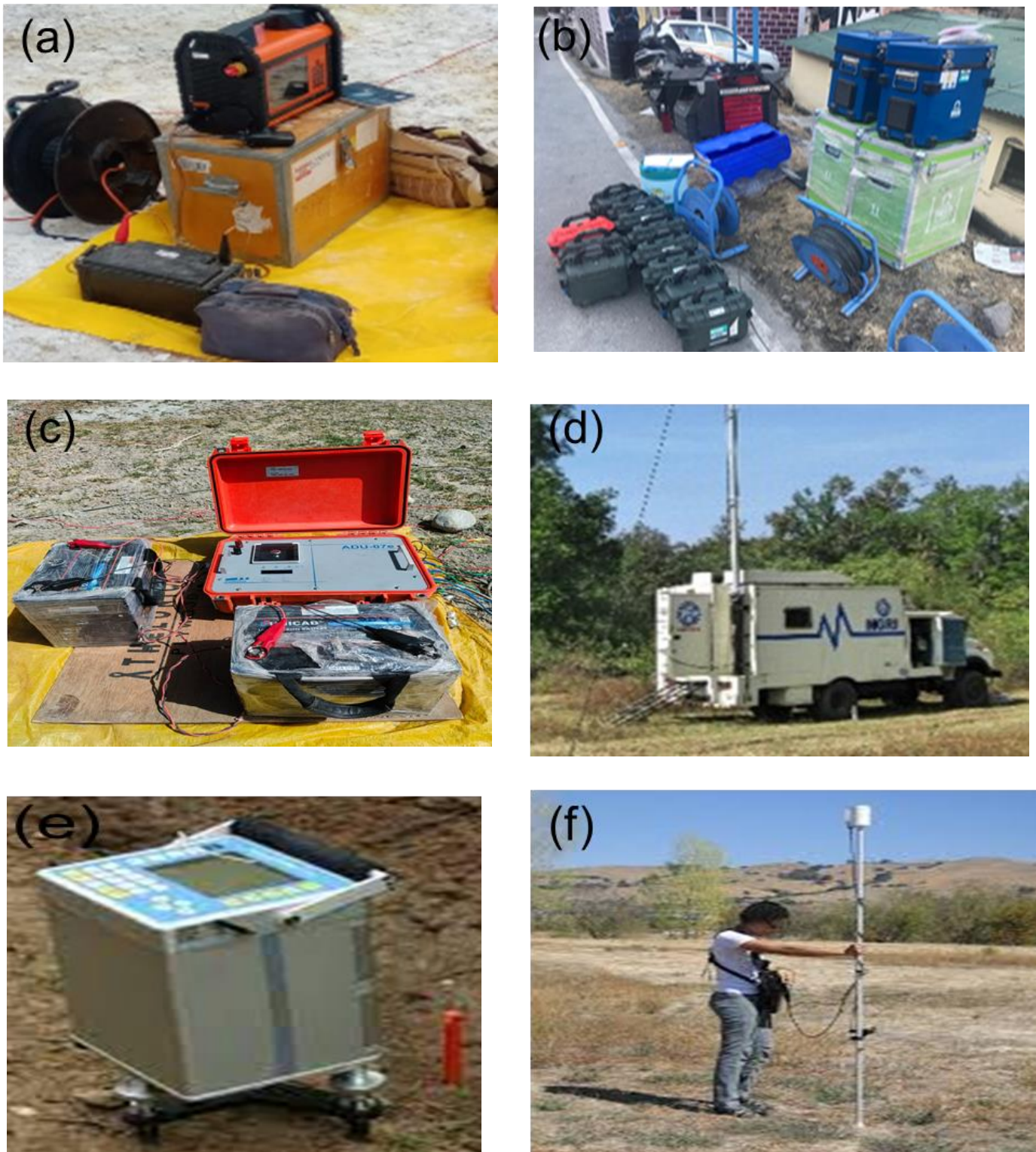
Figure 4. Geophysical field instrumentation set-ups for subsurface investigations in geothermal exploration (a) Electrical Resistivity Tomography (ERT), (b) Electric-field Vector Resistivity Imaging (EVRI), (c) Magnetotellurics (MT), (d) Seismic, (e) Gravimeter, and (f) Magnetometer.
