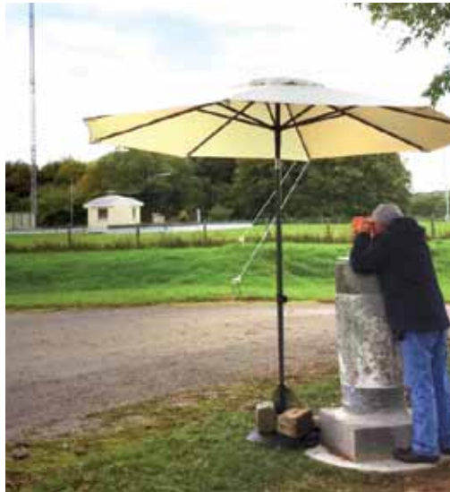
Figure 3. Special set-up for testing the circle graduation accuracy according to the ISO 17123-3 standard
