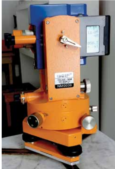
Figure 5. The WIDIF Diflux as a combination of the TDJ6E-NM and the blue magnetometer console, mounted on the telescope. The console also comprises a GPS receiver, a clock, a battery and three LCD displays, one of them being visible here. Note also the second under plate, allowing using pillars fitted with 120° v-grooves.
