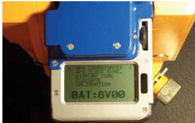
Figure 7. Measurement menu of the WIDIF at switch-on. Note the rocker switch (upper right) allowing to navigate the menu. It is extremely soft to activate and when idle, remains in the same position so as to keep the magnetic signature unchanged.
