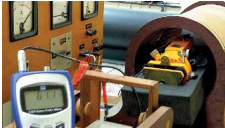
Figure 4. Our set-up for idealization. The reading on the teslameter is in Gauss.
