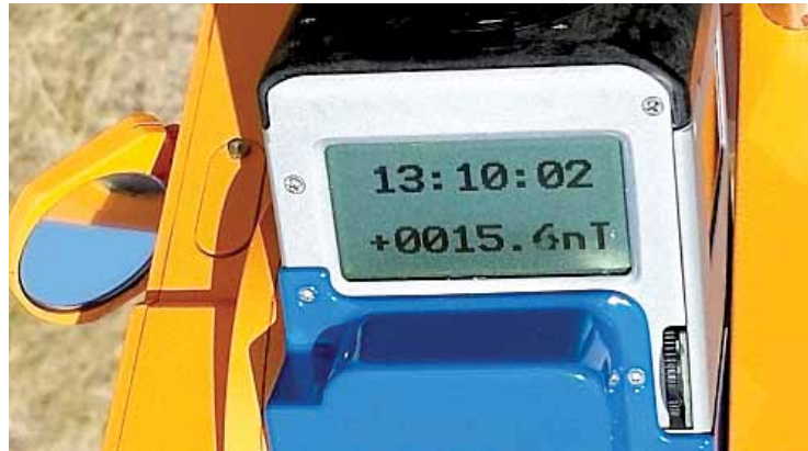
Figure 6. The WIDIF display during a measurement session. The display will change its orientation to fit the telescope position.
