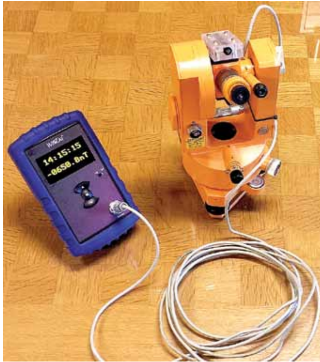
Figure 10. The FLM4/A Diflux electronics. This has the same functionalities as the WIDIF.
