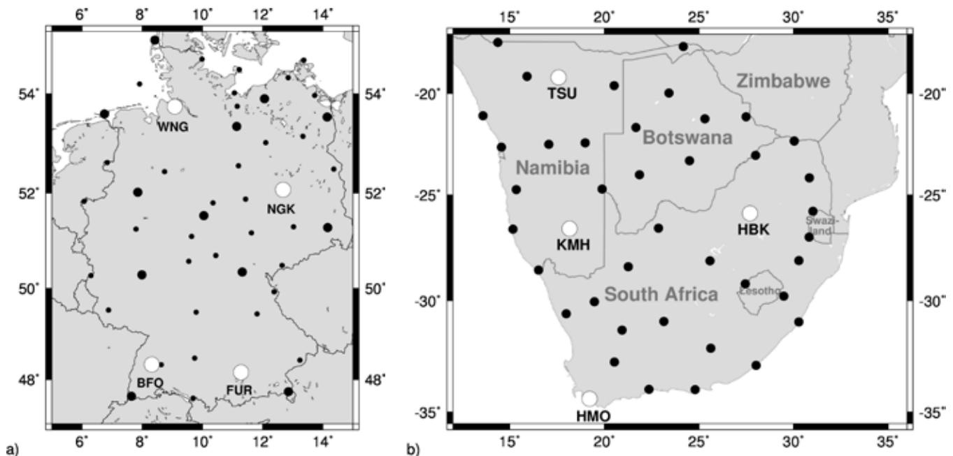
**Figure 1.** Maps of geomagnetic observatory (white dots) and repeat station (black dots) distribution for a) Germany and b) southern Africa. For Germany, large black dots are first order repeat stations with on-site variometer, small symbols are second order stations not considered in this study.
