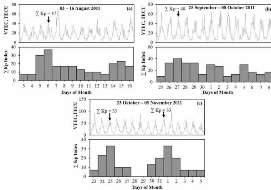
**Figure 6.** (a) Upper panel shows the diurnal variations of GPS-TEC between 3 and 16 August, 2011. The downward arrow indicates the day of occurrence of magnetic storm, the lower panel shows the variations of  $\Sigma Kp$  index for the same period. (b) the same variations as Figure 6a but for the period of 25 September-08 October, 2011. (c) same variations as Figure 6a but for the period of 23 October-05 November, 2011.
