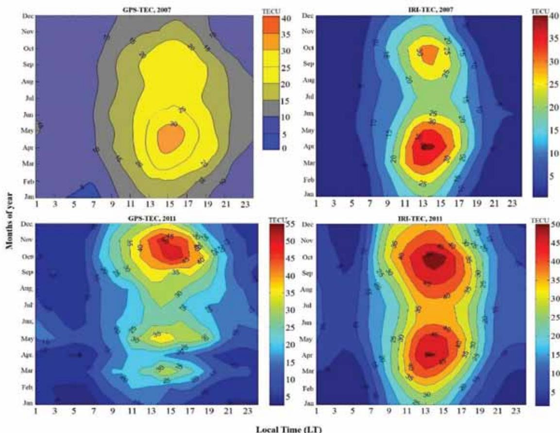
**Figure 1.** Upper panel (left) shows the contour plot of average monthly GPS-TEC variations during period-I (2007) over a low latitude station, Agra, India and the upper panel (right) presents the IRI-2012 model TEC data variations over the same station and for the same period. The lower panel shows the same variations as above but for the period-II (2011).
