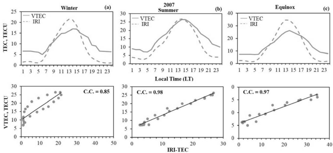
**Figure 2.** Upper panel presents the variation of GPS-TEC and IRI-TEC by solid and dotted lines during each of the three seasons (winter, summer and equinox) respectively for the period-I (2007). The lower panel shows the correlation plots between VTEC and IRI-TEC for the same as above.
