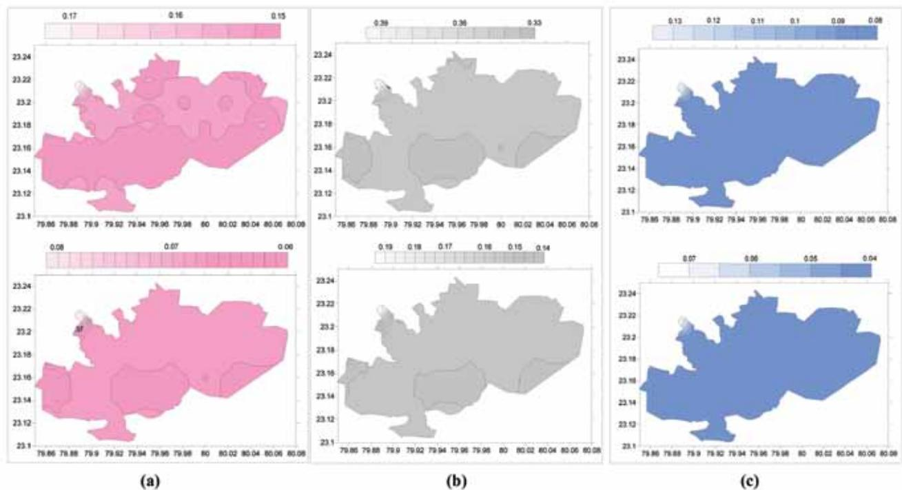
**Figure 6.** (a) Peak Ground Acceleration (PGA) contours for 2500 years (top) and 500 years (bottom) of return periods with an exposure period of 100 years. (b) Short period spectral acceleration values at 0.2 sec for return period of 2500 (top) and 500 (bottom) years with 5% damping for both rock and soil site conditions. (c) Long period spectral acceleration values at 1 sec for return period of 2500 (top) and 500 (bottom) years with 5% damping for both rock and soil site conditions.
