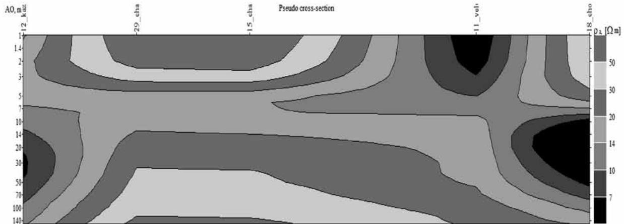
Figure 9. Profile CD Resistivity pseudo cross section.
