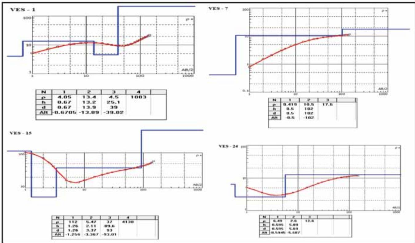
Figure 7. Resistivity curves and tables showing thickness.
