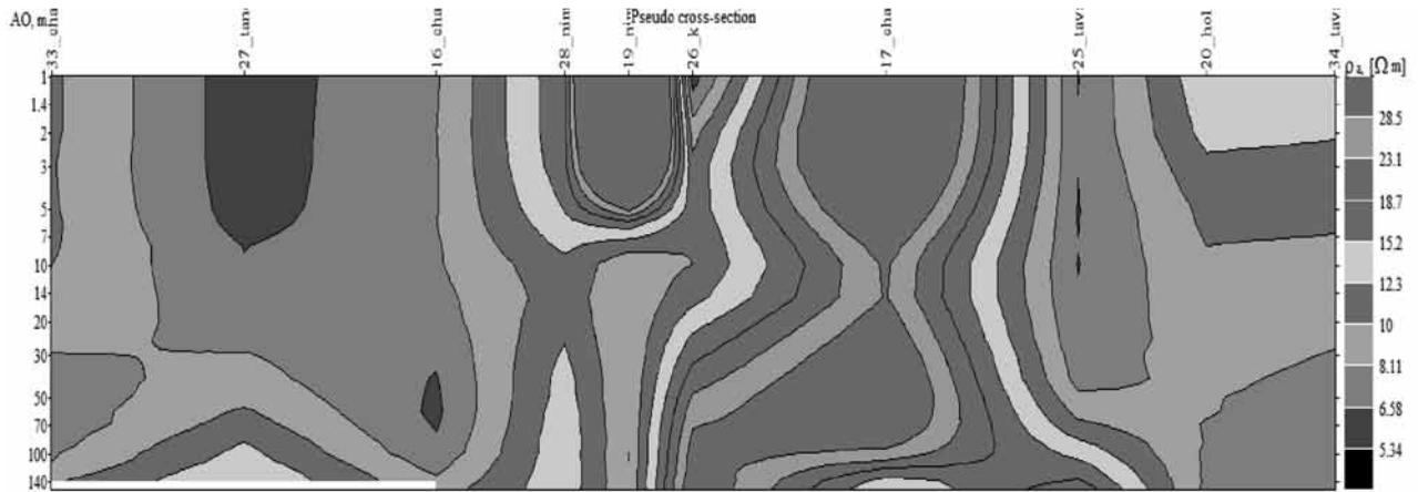
Figure 10. Profile EF Resistivity pseudo cross section.
