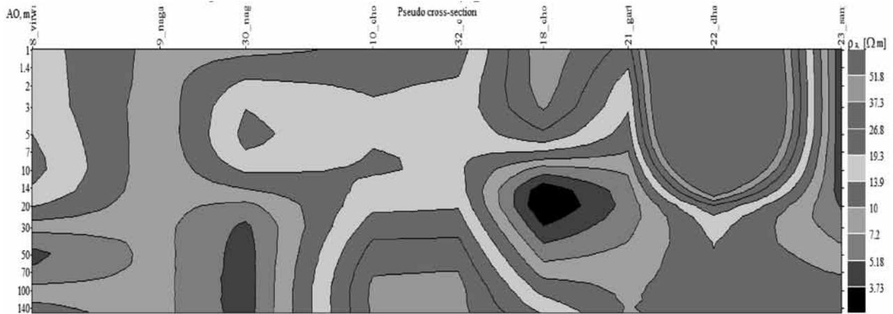
Figure 11. Profile GH Resistivity pseudo cross section.
