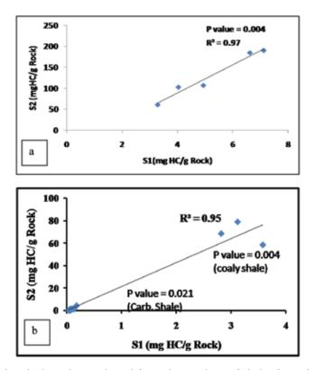
**Figure 3.** Correlation of S1 and S2 hydrocarbons released from the pyrolysis of shales from the (a) Tadkeshwar lignite mine, Surat, and (b) Rajpardi lignite mine, Bharuch, respectively, Cambay basin.
